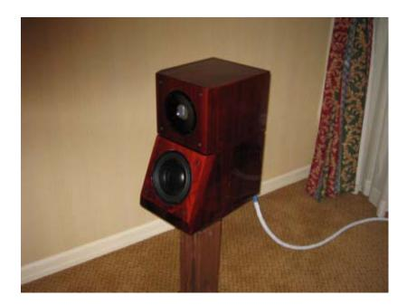
I felt the Orsa monitors, at \$2200 per pair, made some of the best sound I heard at the show. The Orsa's appear to utilize the same or similar ribbon tweeter to that employed by the Sound Fusion speakers, and have a radical two-cabinet design, with the bass-reflex port placed between the two cabinets.
