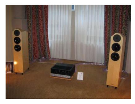
**Butler Audio** was demonstrating its revolutionary Monad monoblock amps with **Escalante Design** monitors. The Butler amps (\$18,995 for the pair) produce 100 wpc of single-ended power through a single 300B output tube per channel. How is this possible? Butler Audio has discovered a means to DC couple the 300B tube directly to the speakers.
