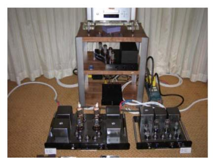
Driving the Orsa's was a massive tube amp employing a 300B tube as a driver and an 805C as an output tube. The amp is said to be good for 45 wpc, and drove the Orsa's to perfection. The best news? The price, at only \$2950. Oh, and did I mention that it can be used as a power amp or as an integrated?
