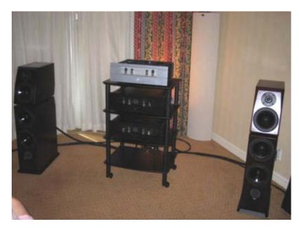
Von Schweikert's VR-4 JR speakers were also in use in the MOSCODE room, who were heralding their return with the introduction of the new 401 HR hybrid amplifier (around \$5000). The amp utilizes a tube driver stage with a Cascode emitter, mated to a MOSFET output stage rated at 200 wpc into 8 ohms. Internal construction was top-notch, and the amp has the flexibility to accept a multitude of small-signal tubes, including 6H30Pi, 6922, 6GU7, 12AU7, etc...
